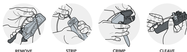
FIGURE 2: Crimp, Cleave, and Leave
