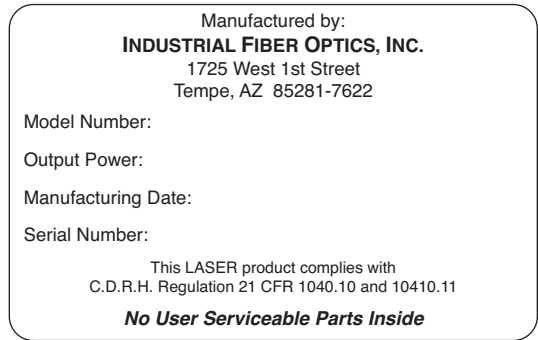
Figure 3. Laser certification and identification label.
